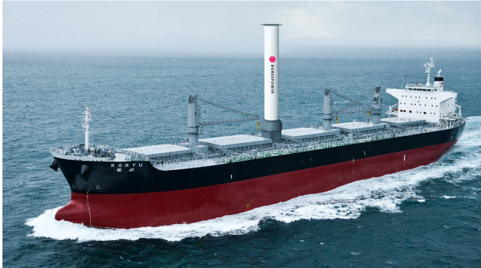
Norsepower's Rotor Sail, with a tilting foundation, will replace one of the deck cranes in a first-of-its-kind installation onboard MV Koryu
